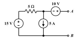
Determine the Thévenin equivalent circuit with respect to terminals A and B.
